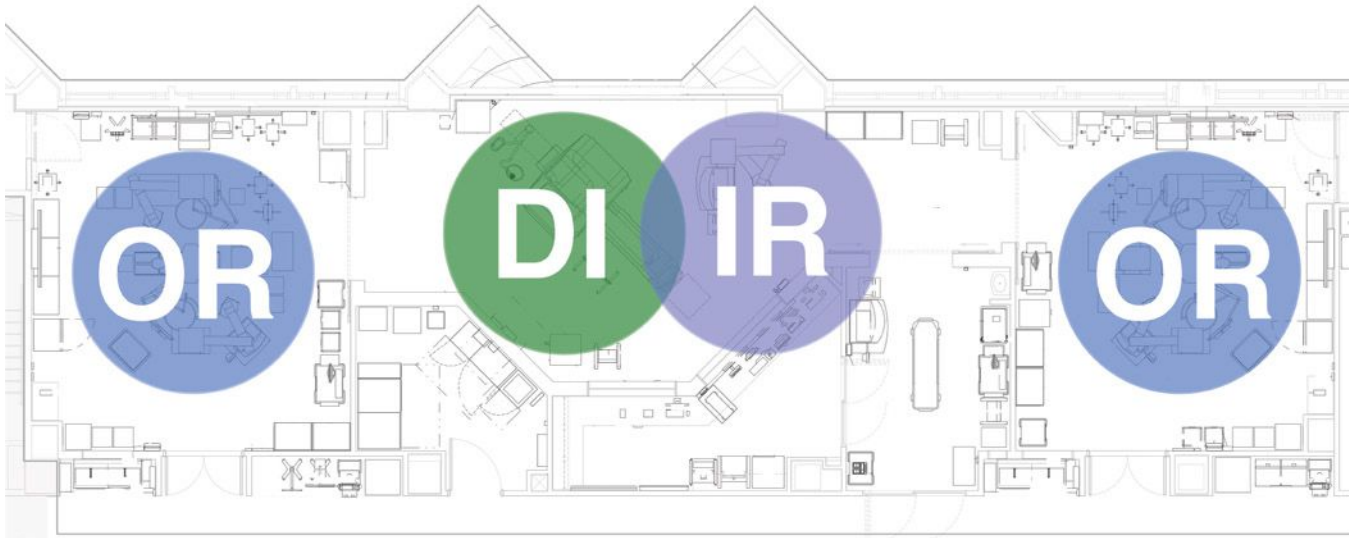
A hybrid suite showing operating room (OR), diagnostic imaging (DI) and interventional radiologist (IR) areas.
